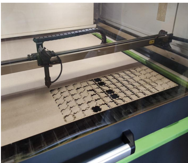
Fig.14. Laser Cutting of the MDF Material.
