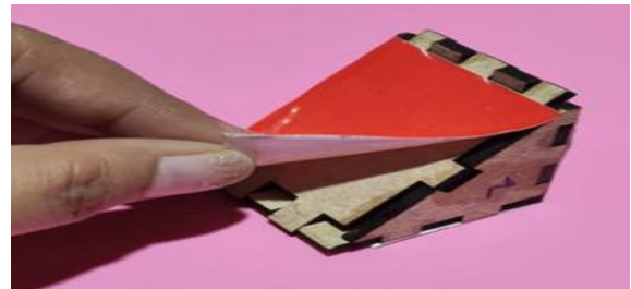
Fig. 33. Placing of the Colored Vinyl Stickers in the Triangular Prism Pattern.
