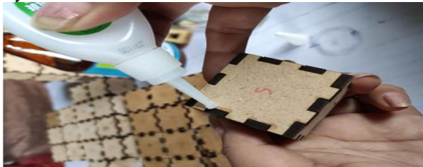
Fig. 27. Application of Adhesive at the Edge of the Cube Patterns
