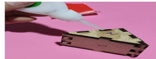
Fig. 28. Application of Adhesive at the Edge of the Triangular Prism Patterns.
