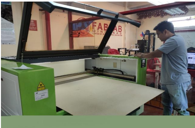
Fig. 13. MDF Material Ready for Laser Cutting
