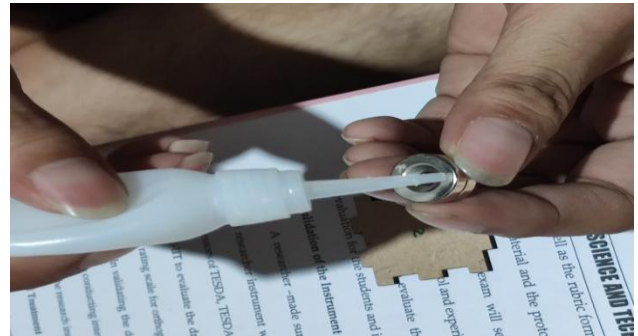
Fig. 22. Applying Adhesive to the Magnets
