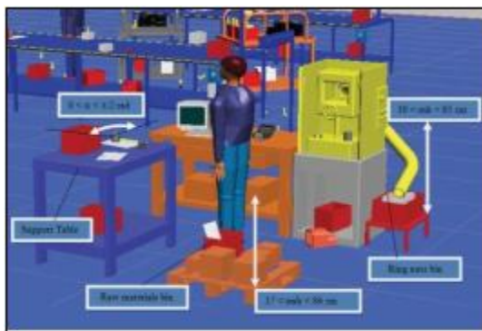
Fig.2. Actual configuration of the Seal Press workstation (with design parameters).
