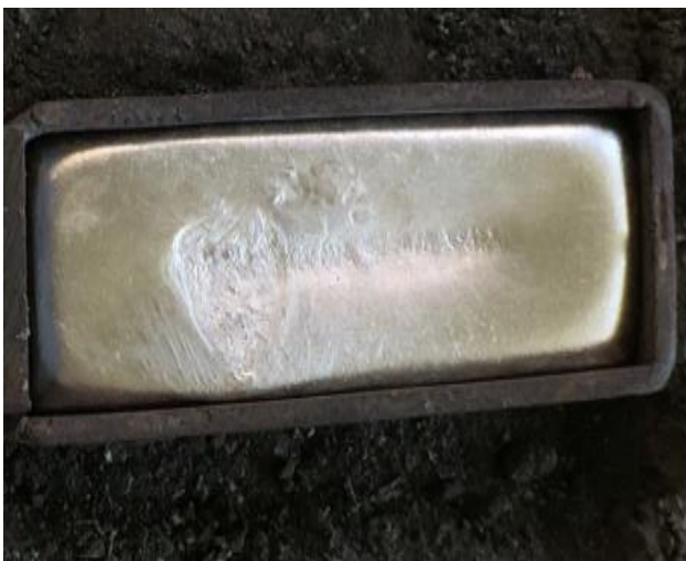
Fig 4.6. Cast and mould after casting.
