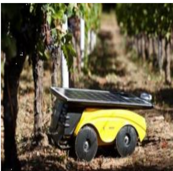
Fig. 3.2: Solar Robot Used In Vines to Cuts Grass and Weeds.
