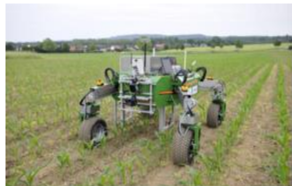
Fig: 1.1: Navigation System of the Autonomous Robot Boni Rob.
