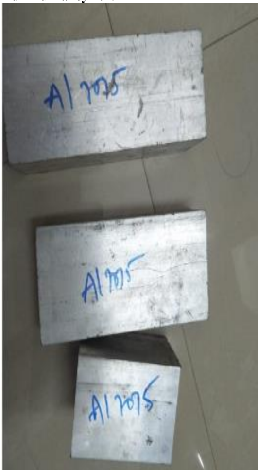
Fig .2 . Materials of Aluminum alloy 7075.
