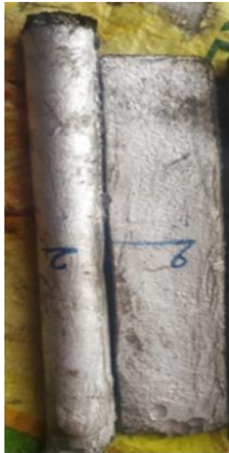
Fig. 8. Composition Aluminum alloy 7075 + Gr 8%.
