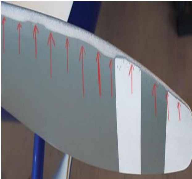
Fig.3. Corrosion Areas and Damaged can be repaired with Cold Spray Technology (stocktonpropeller.com).
