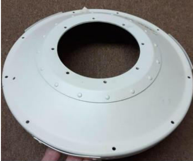
Fig.5. Spinner Bulkheads can be repaired with Cold Spray Technology (stocktonpropeller.com).
