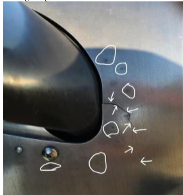
Fig.4. Propeller Spinner Dome damage can be repaired with Cold Spray Technology (Backcountry Pilot).
