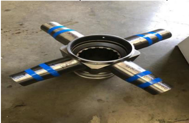
Fig.6. Steel Hub and Aluminum hubs-Both can be repaired with Cold Spray Technology (stocktonpropeller.com).
