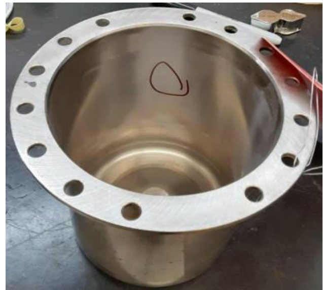
Fig.7. Propeller Cylinder Wear and Tear can be repaired with the Cold Spray process (stocktonpropeller.com).
