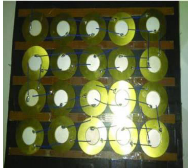
Fig.4. Series and Parallel connected sensor.
