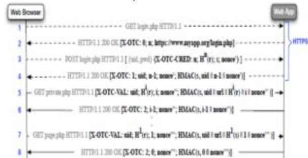
Fig. 7. Flow diagram of a web session authenticated with OTC. Messages 1 to 4 show the OTC setup phase and messages 5 to 8 show the OTC authentication phase. Each HTTP request and response include an OTC header with protocol information.
