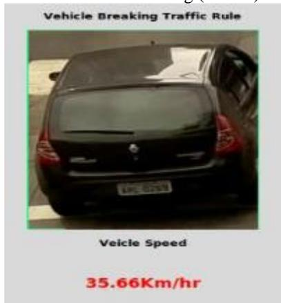
Fig .A.Vehicle violation capture and speed calculation.
