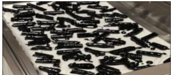
Fig.3. Encapsulation of cigarette butt with bitumen
