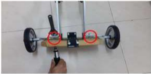
Fig-6: Attaching the base to the bicycle frame
