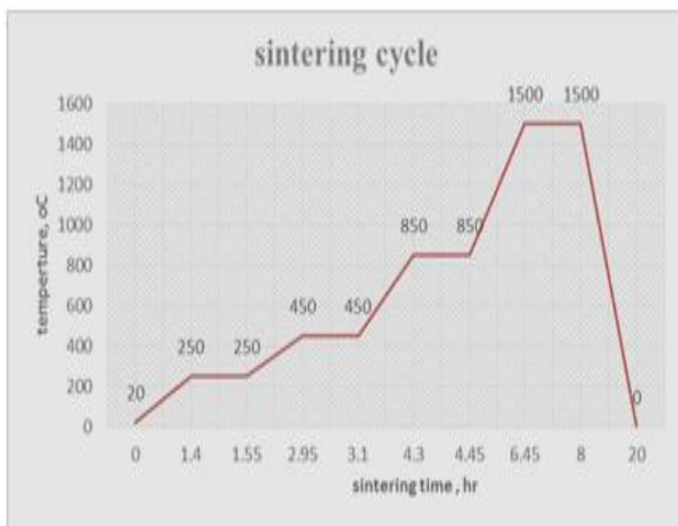
Fig.2 Sintering cycle for tungsten heavy alloy version no 7, sintered at 1500 oC.
