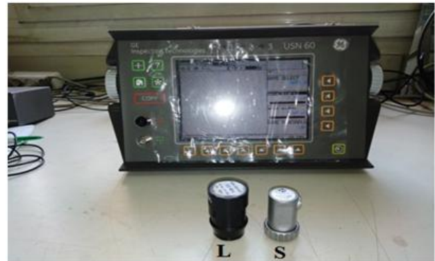
Fig.3. The ultrasonic flaw detector device (USN 60 model), with Longitudinal (L) and Shear (S) Probes.
