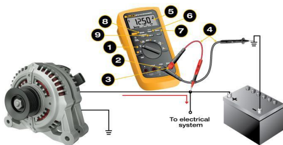
Fig 1 dc voltage with a digital multimeter.
