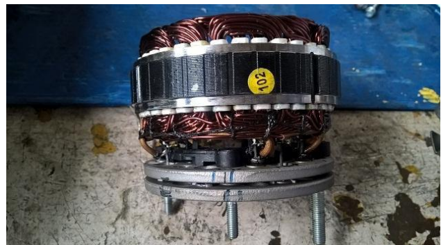
Fig 5 In multimeter checking, short circuit between W to Ground in the alternator.
