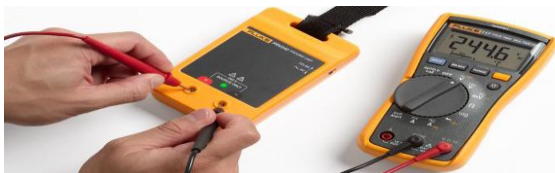
Fig 2 electrical test tool operation with a proving unit.
