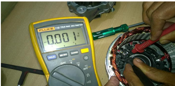
Fig 6 In multimeter checking, short circuit between W to Ground in the alternator.
