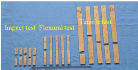
Fig 5 Digital images of short fiber composite specimens (35wt%) used for the impact, flexural and tensile tests.
