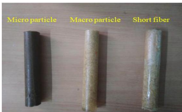
Fig 10 Digital image of the composite rod for micro, macro particle and short fiber reinforced with epoxy composites
