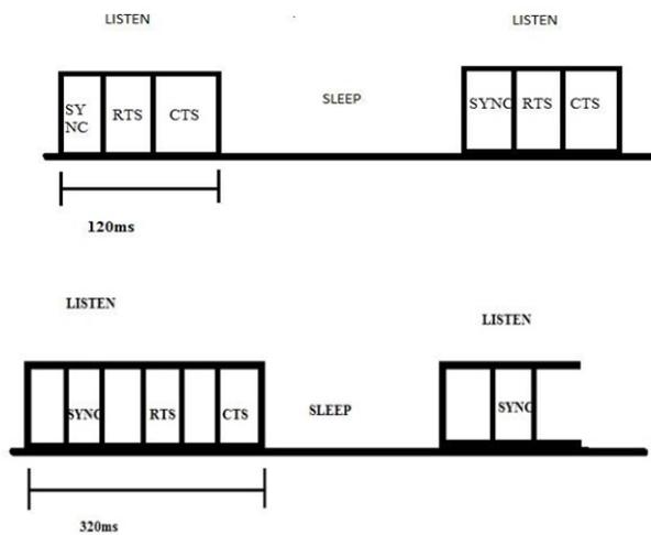
Fig.2. Modified S-MAC schedules to accommodate large propagation delay. (a) Shows the listen window length currently implemented in Tiny OS. (b) Shows increased listen window to accommodate propagation delay of each packet.
