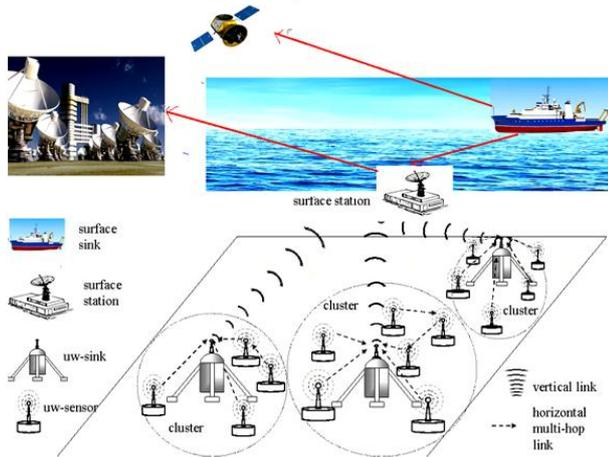
Fig.2. Architecture for 2D Underwater Sensor Networks.
