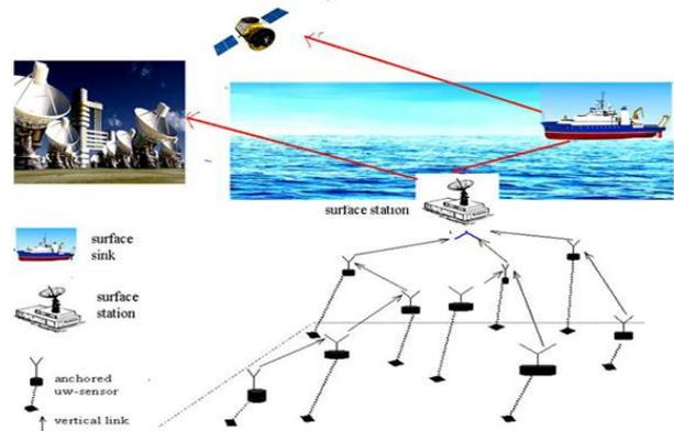
Fig.3. Architecture for 3D Underwater Sensor Networks.
