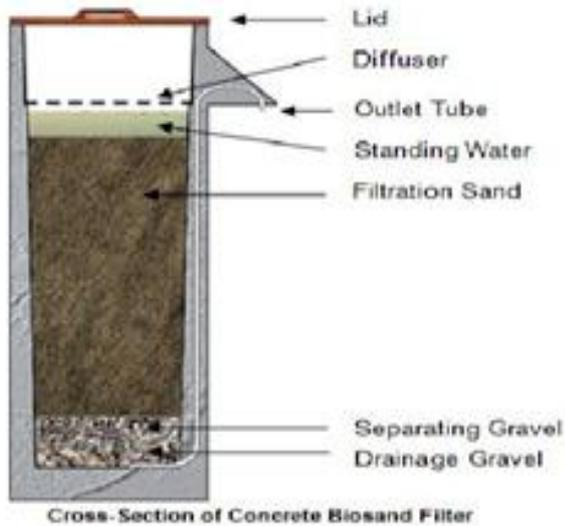
Fig.1. Biosand Filtrations Process.
