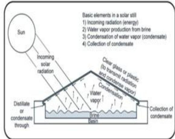
Fig.2. Desalination Process.
