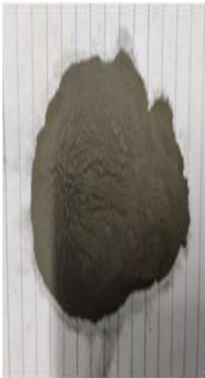
Fig.4. AL7068 40 \mu size powder.
