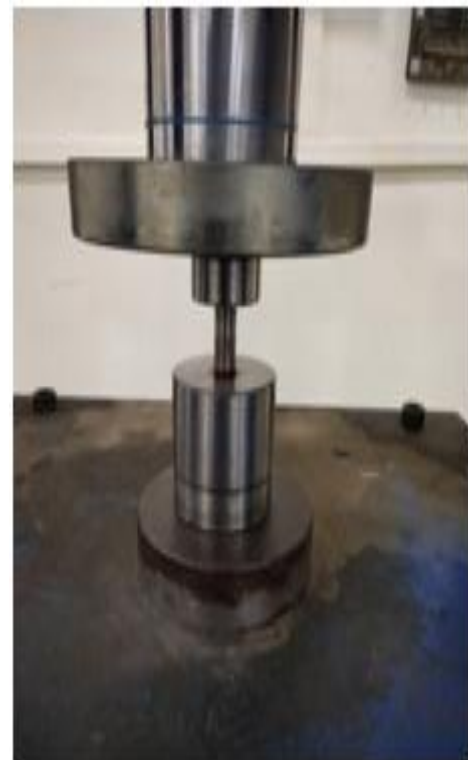
Fig.2. Compacting of sample using Digital hydraulic press.
