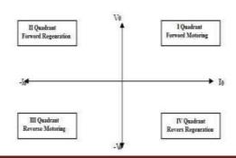
Fig.1 Basic operation of Four quadrant chopper.
