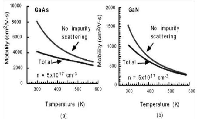
Fig. 3 (a) Temperature vs mobility for GaAs HEMT (b) Temperature vs mobility for GaN HEMT.
