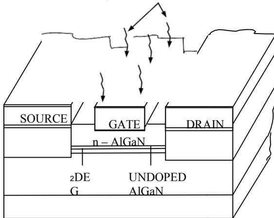
Fig .2 Basic construction of HEMT.
