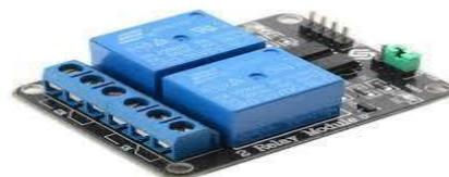
Fig.5 Relay Module.
