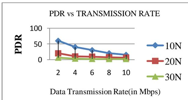
Fig.6 PDR Vs Data Transmission Rate.
