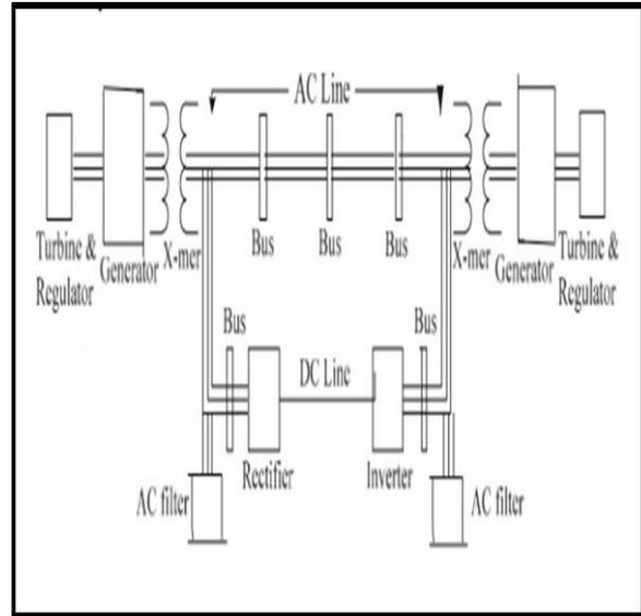
Fig.1 Block Diagram of Proposed AC-DC Transmission Network.
