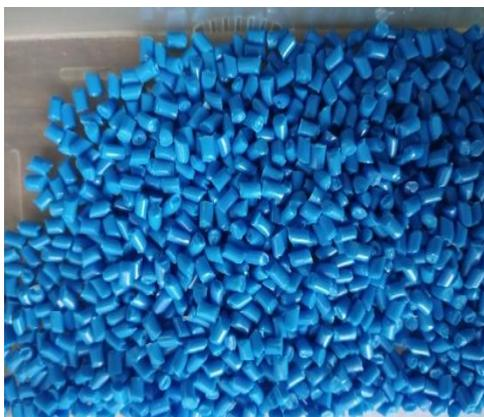
Fig.2 Raw material-Poly propylene.
