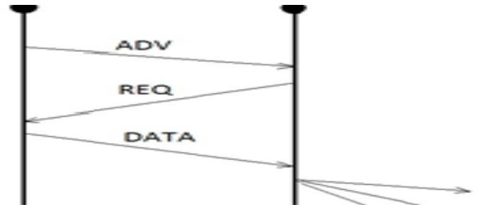
Fig1. Sensor protocol for information via negotiation (SPIN).
