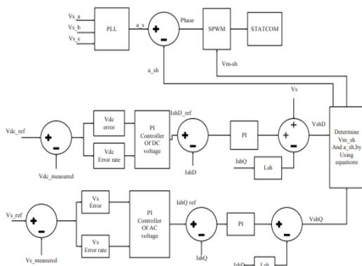
Fig.3 D-Q axis based STATCOM controller.
