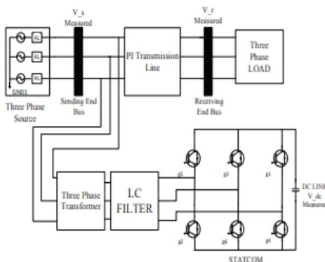
Fig. 2. Schematic diagram of STATCOM connected to power system
