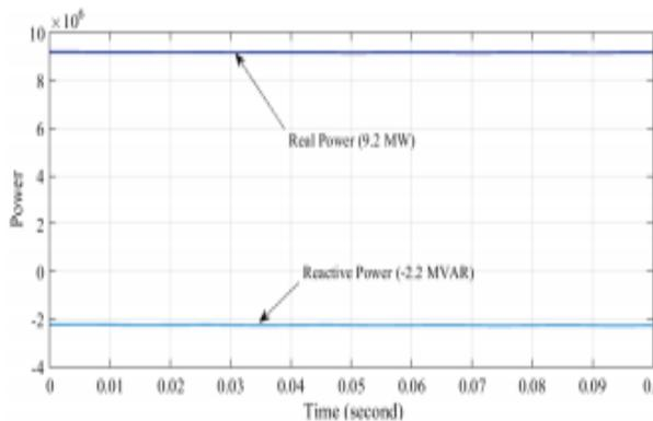
Fig.6 Real and Reactive Power (Without STATCOM)
