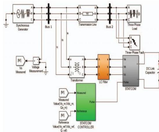
Fig.4 Simu link Model of STATCOM connected Power System.
