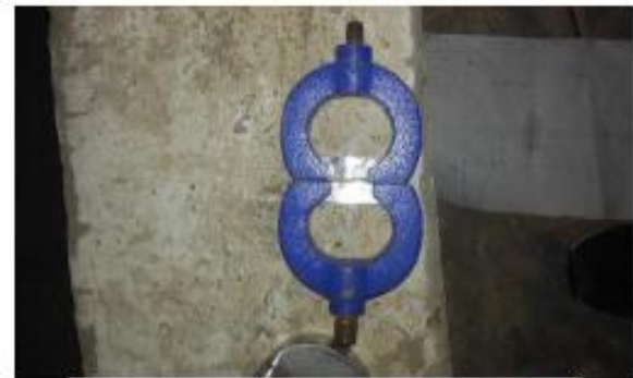
Fig.4 Load delivering tool for compressive test.
