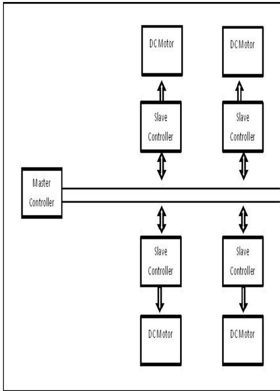
Figure1: Synchronized Motor Controller
