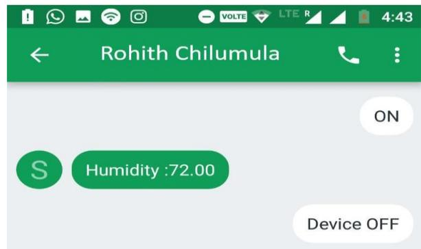
Fig.9 (We can switch OFF the system any time by sending a SMS message “Device OFF”).
