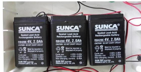
Fig.6 4V Lead Acid Rechargeable Battery Connected in Series.
