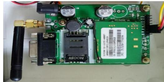
Fig.2 GSM Module.
