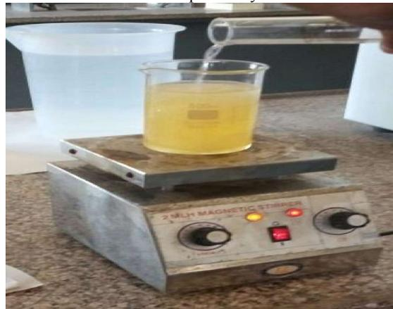
Fig.3 Mixing of Methanol into the Soya bean oil.
