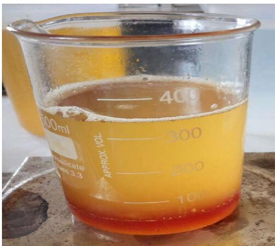
Fig.4 Separation of Bio-diesel and glycerine.
