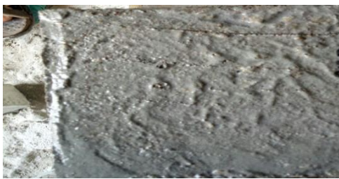
Fig.13 20 ml inoculum + 10 g calcium Lactate 1 day shaking.
