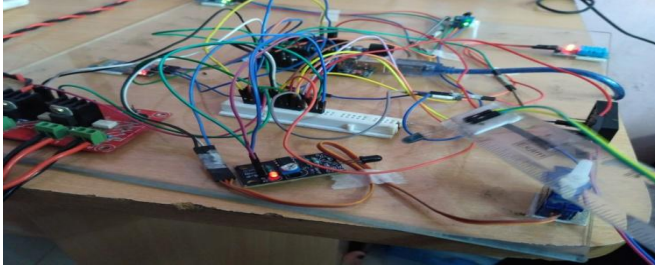
Fig.4 IR Communication to detect chair is not at exact position.
