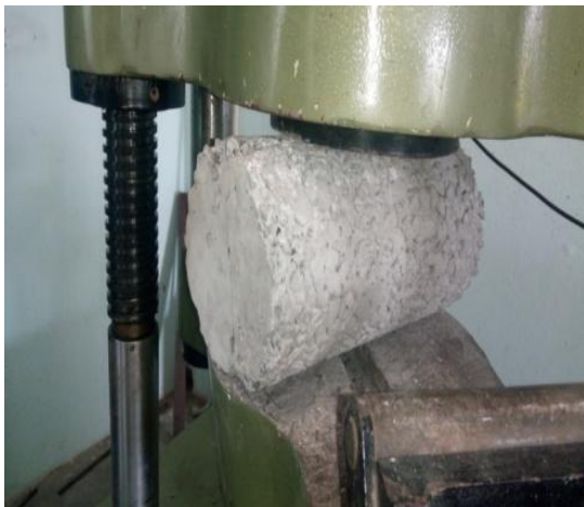
Fig.7 Split Tensile Strength Test.
