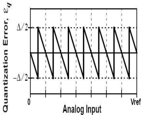
Fig.3 Error at the DAC output (from an ideal ADC-DAC series connection). The error comes purely from the quantization error of the ideal 3-bit ADC.
