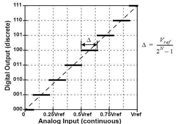
Fig.2. Transfer functions of an ideal 3-bit ADC. For an N-bit ADC there are 2N output levels corresponding to input voltage ranges of width  $\Delta$ .
