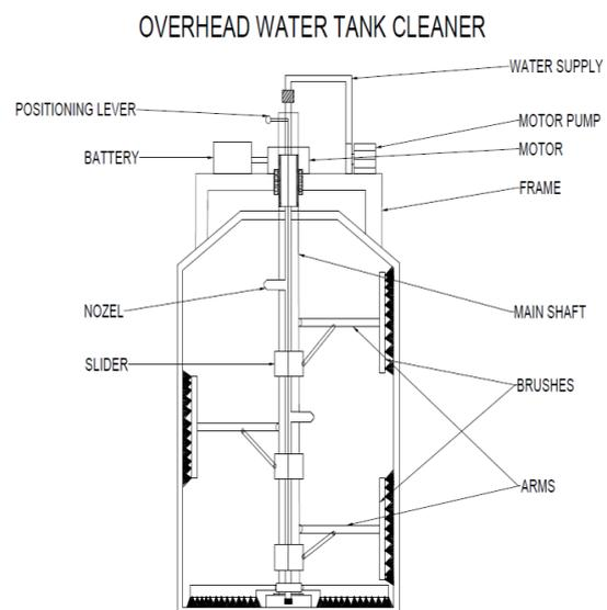
Fig.8. Overhead water tank cleaner
