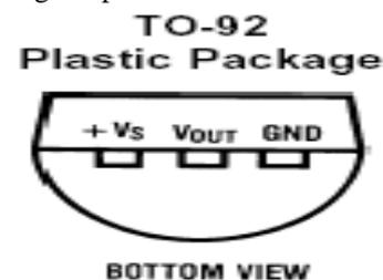
Fig8 Pin Diagram of LM 35
