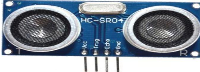
Fig. 11 HCSR-04 Ultrasonic Sensors.
