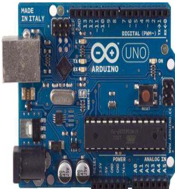
Fig.6 MEGA328 Microcontroller Board
