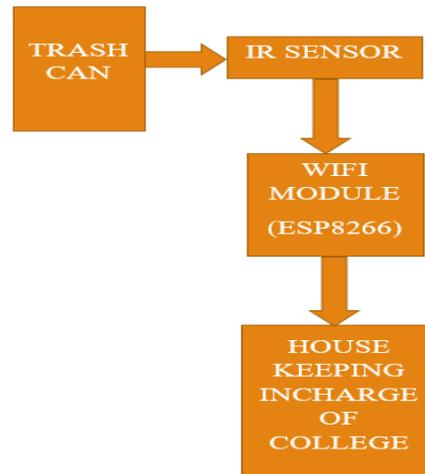
Fig. 1 Block diagram for a Garbage Level Monitoring System.
