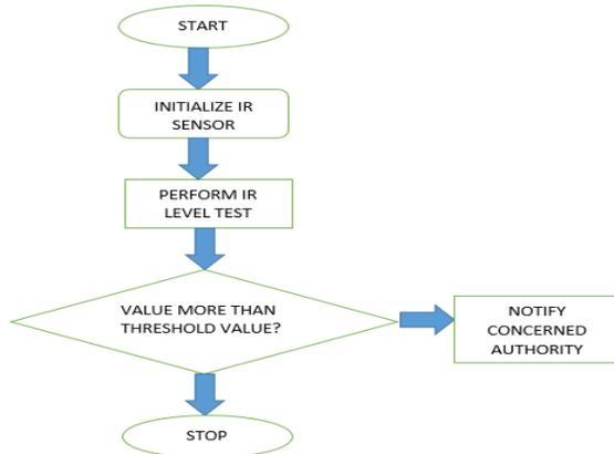
Fig. 2 Dataflow diagram for garbage monitoring system.
