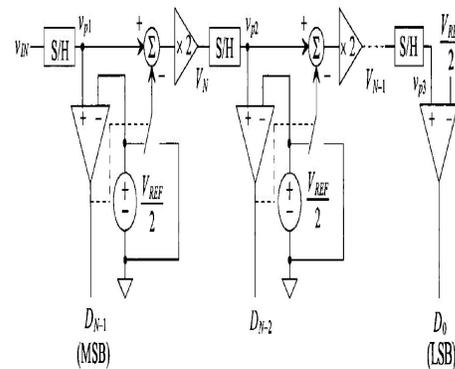
Fig 1 pipeline A/D converter
