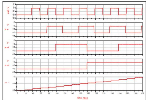
Fig 4 Simulation Results for Pipeline ADC
