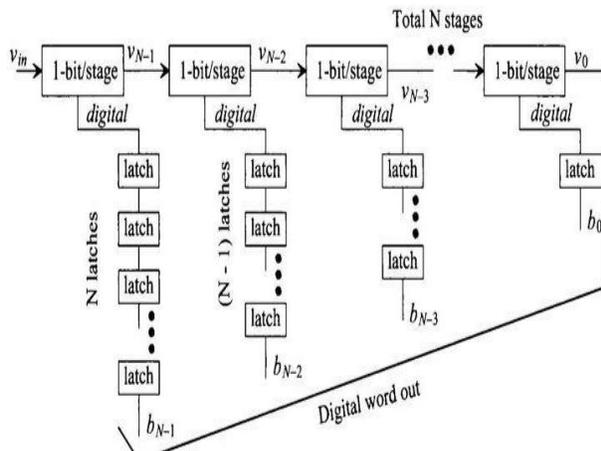
Fig 2. Pipeline ADC based on cyclic stages.
