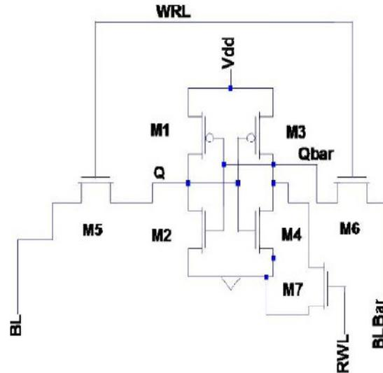
Fig.6 Fully differential 7T SRAM cell[9]
