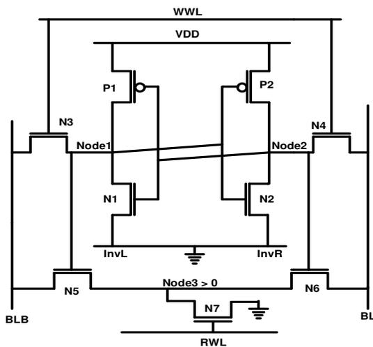
Fig.2 9T SRAM Cell[11].
