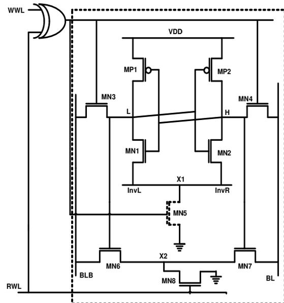
Fig.3. Fully Differential Low Power 10T SRAM (LP10T)[12]
