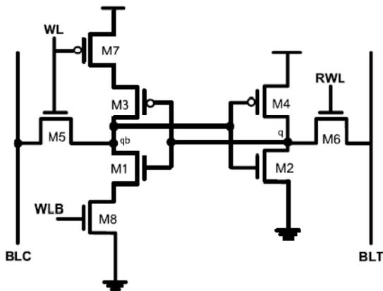
Fig.5 Write-And-Read-Enhanced 8T SRAM cell (WRE8T)[14].
