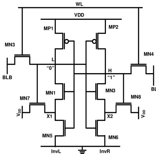
Fig.4 Schmitt trigger based 10T SRAM cell (ST10T)[13]
