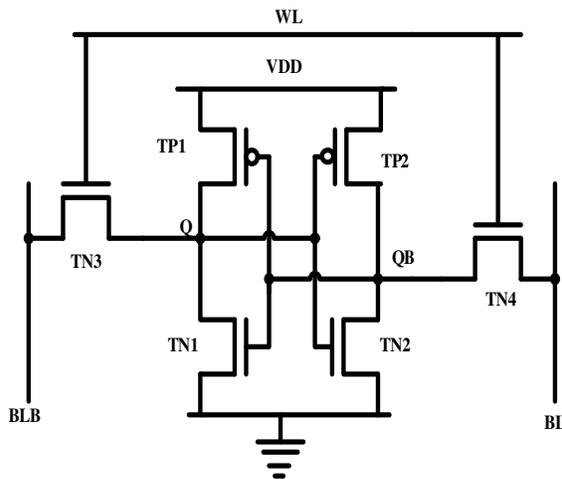
Fig.1 Conventional 6T SRAM cell[10]
