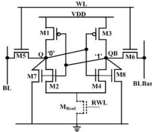
**Fig.7** Proposed Differential 8T SRAM Cell
