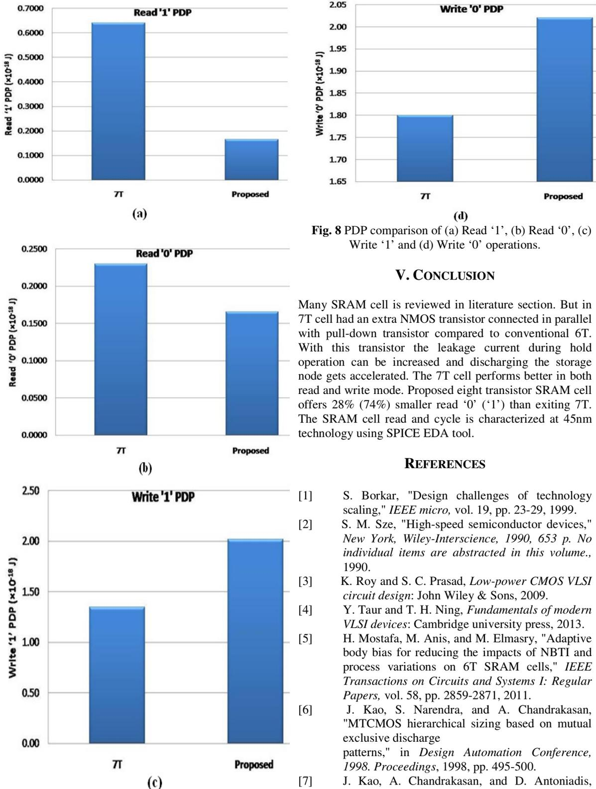
Fig. 8 PDP comparison of (a) Read '1', (b) Read '0', (c) Write '1' and (d) Write '0' operations.
