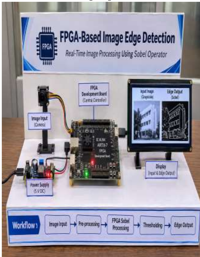
Figure 1: FPGA-Based Image Edge Detection System Using the Sobel Operator
