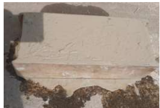
Figure 16 :Casted brick mould
