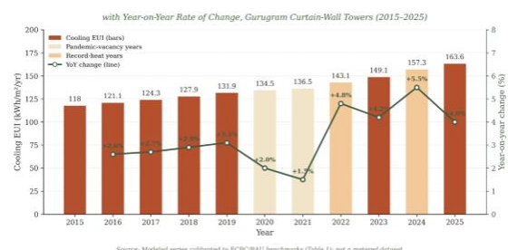
Figure 3. Modeled cooling-specific energy consumption (EUI) with year-on-year rate of change, Gurugram curtain-wall office towers, 2015–2025.
