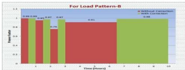
Figure 14: Power Factor Variation for Load Pattern B
