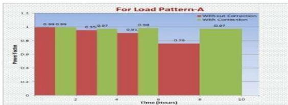
Figure 13: Power Factor Variation for Load Pattern A
