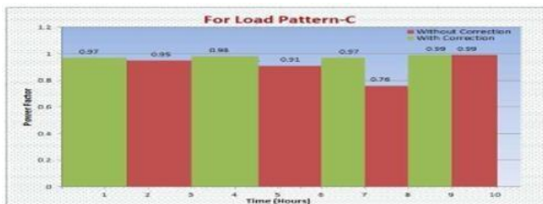
Figure 15: Power Factor Variation for Load Pattern C
