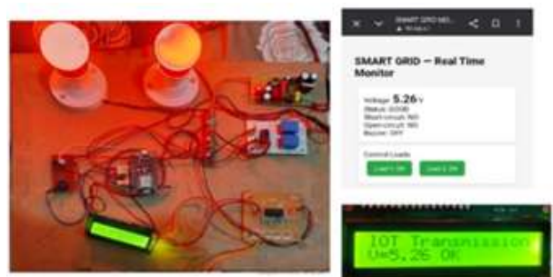
Fig 5. During under voltage condition
