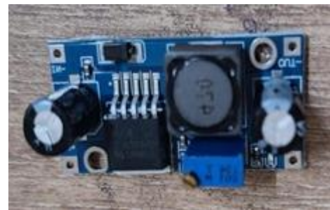
Fig.3 Charge Control Buck Booster
