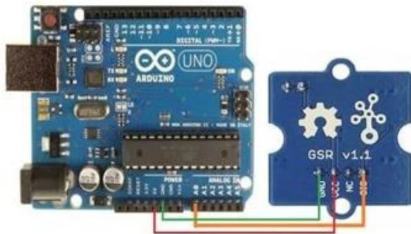
Fig. 4. GSR sensor interfaced with Arduino UNO.
