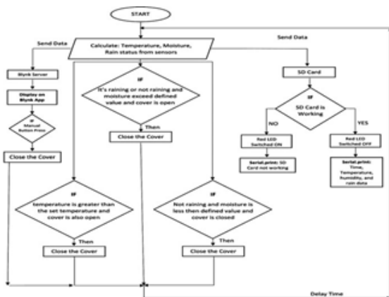
Figure.2. Methodology workflow of the Voice-Enabled IoT Irrigation for Smart Agriculture
